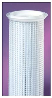
sewn seams. The microfiber material is sandwiched between two flow-enhancing polypropylene mesh screens, then pleated. The cartridge bottom and top sealing ring are made of solid molded polypropylene and are welded to the ends of the pleated cylinder without the use of adhesive. The sealing ring is a pliable gasket, increasing the efficiency and integrity of the seal. THE PL SERIES HAS 25 SQ. FT. OF SURFACE AREA.
